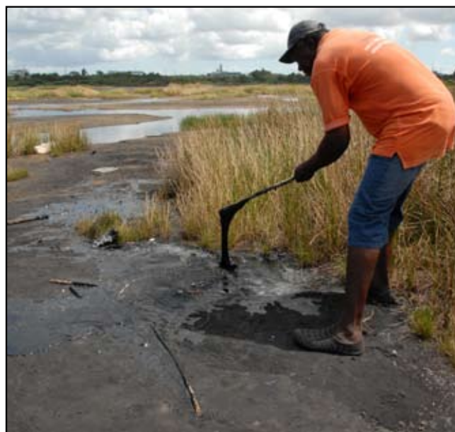
Sampling the tar, with a wooden stick dipped into the sticky fluid asphalt lying just beneath the rubbery crust that forms the fairly stable surface.
